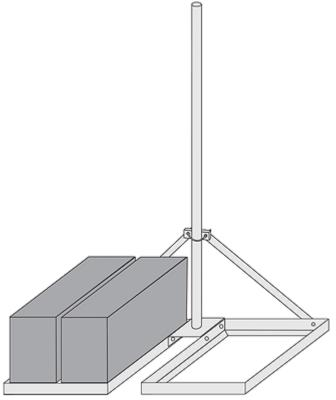
The frames have to be ballasted with concrete blocks (shown on one side)
