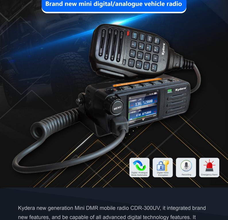
supports both digital analogue working modes. Features: ◆ True-2-slot: Provide 2-slot communication which allows for 2 talk paths on a frequency; comply with MotoTrbo Tier I&II. ◆ Support both digital and analogue modes, fantastic digital operation, and secure the smooth transition from analogue to digital, and improve the radio utilization. ◆ To adopt the TFT color display, convenient operation. ◆ Be capable of definable keys to convenient for accessing common fucntions.
