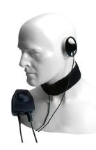
The CXR16 incorporates a high performance bone conductive throat vibration microphone that provides clear audio transmission even in the noisiest of environments. Unlike conventional headsets, the bone conductive throat mic is not adversely affected by external sounds.
