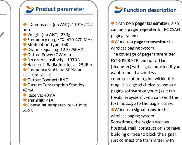
power adapter and fix it in a suitable place, then it work as a signal booster. It is so simple to boost the range of communication.
