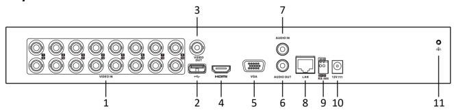
\*: The rear panel of iDS-7208HQHI-M2/S and iDS-7232HQHI-M2/S provide 8 and 32 video input interfaces.
