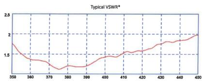
\* VSWR shown is AFB-S1 on a 1x1m (3'x3') ground plane with 5m of CS23 (RG58 c/u) cable
