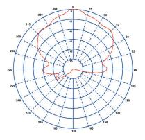
Patterns measures on a 600x600mm (2'x2') ground plane without cable
