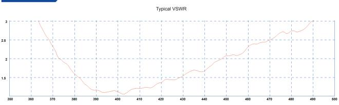
\* Measured on a 600x600mm (2'x2') ground plane with 1m (3') of low loss cable
