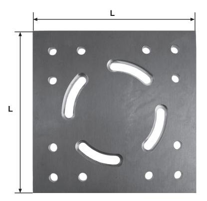
**TP** mechanical tilting plate allows, depending on the mounting orientation, a mechanical down or up tilting up to 45 degrees. The tilting angle is continuously adjustable. It can be also used to adjust the antenna orientation on horizontal plane when the antenna is mounted on a horizontal pole.
