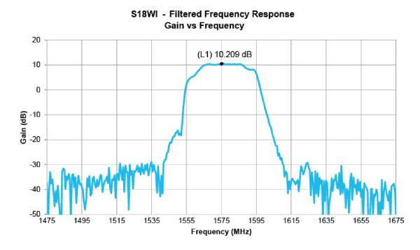
Figure 2-7. Frequency Filtered Response
