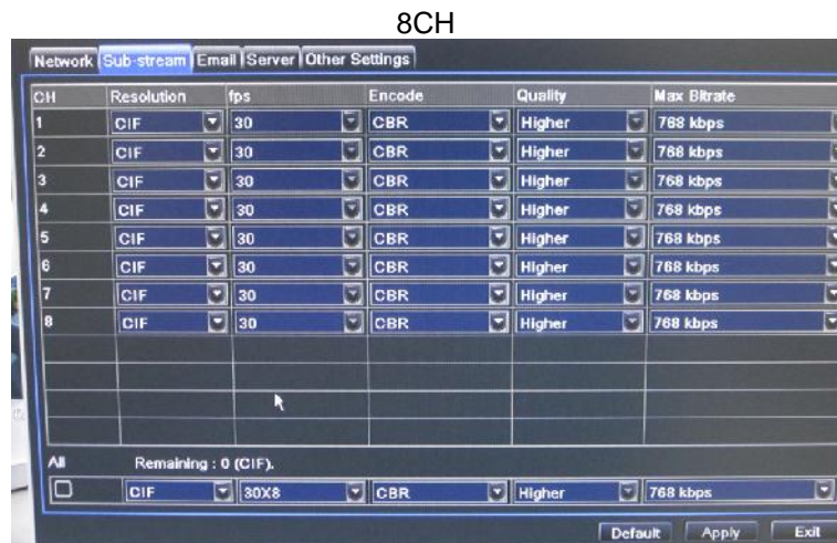
Fig 4-32 network configuration-sub stream
