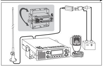
It is very important to select a good quality high efficiency 27MHz antenna. A poor quality antenna or one not designed for the 27MHz band will give very poor performance and could cause damage to the transceiver.
