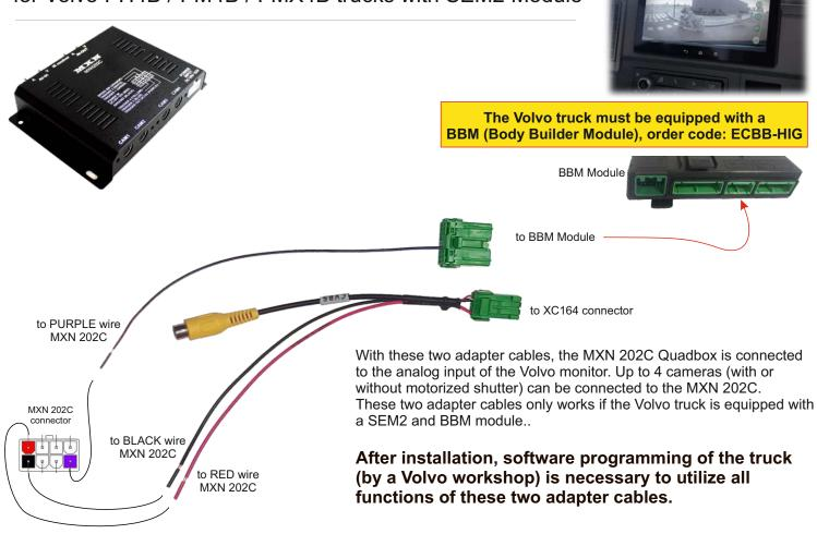
Location of the 5-pin green XC164 connector and BBM Module is under the fuse box in the center of the dashboard
