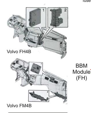
1. Body Builder Module (BBM) 2. Fuse and relay box BBM
