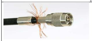
4. Insert the end of the cable thus prepared as far as the stop (click) into the plug housing. Twist the copper braid at right angles.
